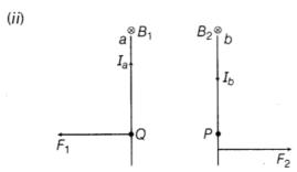
Now, let the direction of current in conductor b be reversed. The magnetic field B2 at point P due to current Ia flowing through a will be downwards. Similarly, the magnetic field B; at point Q due to current Ib passing through b will also be downward as shown. The force on a will be, therefore towards the left. Also, the force on b will be towards the right. Hence, the two conductors will repel each other as shown.
