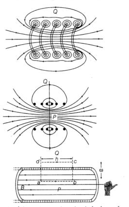
Applying Ampere's circuital law for the rectangular loop *abcd*,
